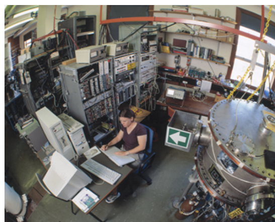
Figure 58: Picture showing the electron scattering from atoms apparatus.
